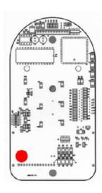
▶ Open the In eXam control unit, and adjust with potentiometer P1.
