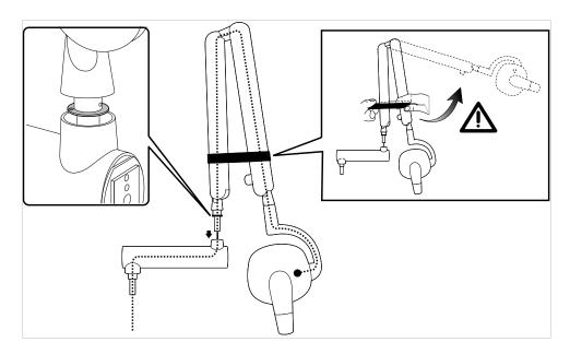
► Completely attach the extension arm with the bearing bushing onto the scissor arm pivot pin, making sure that the nylon ring is in the correct position.
